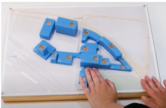
Tactile map made with 3D printer for blind people https://dl.acm.org/doi/10.1145/3173574.3173772
